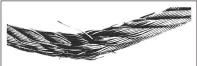
**Reverse bending.** Running this rope over one sheave and under another caused fatigue breaks in wires.
