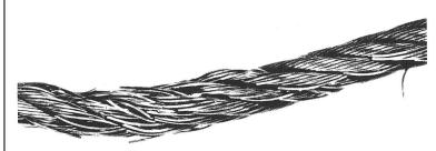
**Undersize sheave grooves.** Sheaves were too small, causing strands to pinch. Wires then fail in the valley between the strands.
