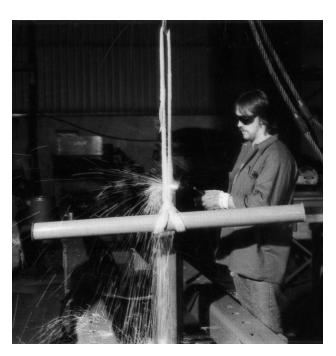
rope or chain slings might scratch the load causing expensive rework. Fire exposure testing was performed by the Offshore Certification Bureau and the product was identified as being as good as wire rope or chain for use in off shore applications in the oil industry.
