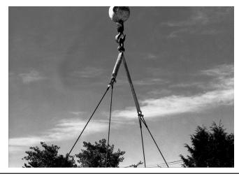
Sling can fail if damaged, misused or overloaded. Inspect before use. Damaged sling shall not be used. Use only if trained. Do not exceed rated capacity. Protect sling from being cut by load edges, corners, protrusions and abrasive surfaces. Avoid exposure to acid, alkali, sunlight and temperature over 180°F. DEATH or INJURY can occur from improper use or maintenance.
