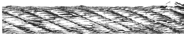
**Lack of lubrication.** Premature breakage of wires resulted from "locking" of strands, which was caused by insufficient lubrication.
